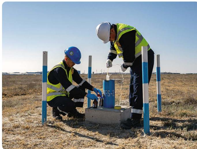
Groundwater samples are collected from 136 observation wells located near the industrial facilities at Tengiz and Korolev fields, as well as from 11 background wells installed at a distance from the production facilities.
